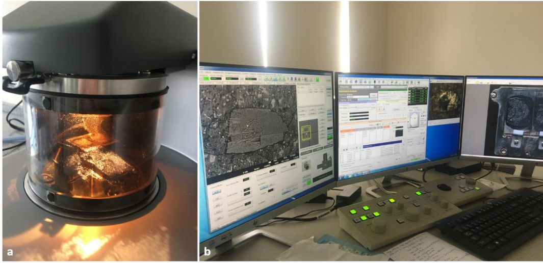
Figure 4.3. a. Carbon coating procedure, b. EPMA system in YEBİM laboratories of Ankara University
