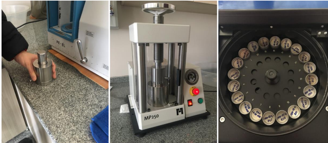
Figure 4.4. Pellet preparation procedure for XRF analyses
